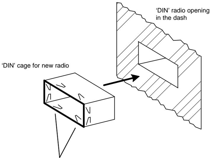
When the 'DIN' cage is inserted into the 'DIN' rectangular opening in the dash, bend these tabs behind the opening in the dash to secure the 'DIN' cage to the dash.
