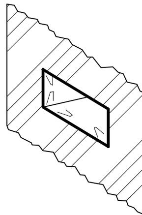
New radios 'DIN' cage slid into the 'DIN' opening of the dash with its tabs bent securing the cage to the dash.
