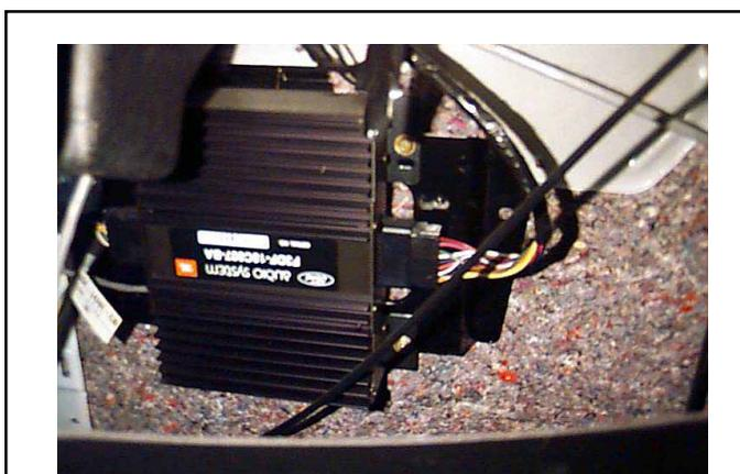
Unplug the both black plastic wire harness connectors that plug into the black colored amplifier in the trunk. One connector on each side of the amp.
