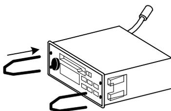
In order for the radio to be removed, clips attached to the side of the radio must be moved inward so the radio can slide out of the dash. Insert the keys and push each key out, away from the radio. The ends of the keys will press into the clips. While pushing the keys outward, pull and the radio should slide forward out of the dash.
