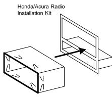
'DIN' Sleeve From New Replacement Radio
