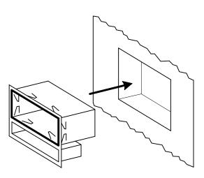
Push The Kit Into The Dash Opening. Depending Upon The Kit Design, The Kit Should Secure To The Dash By Snapping Into The Opening.
