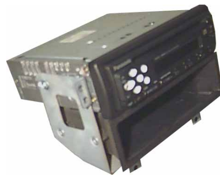
New radio attached to the metal brackets and pocket below the radio
