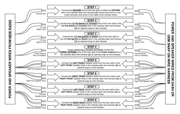
The Install Doctor STRONGLY recommends using a snap on wire harness adapter when installing and wiring a new replacement radio.
