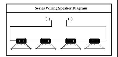
To Calculate The Total Resistance Of A Series Circuit:
