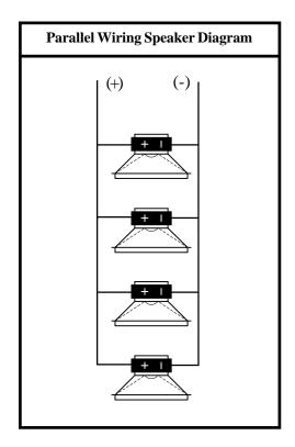
To Calculate The Total Resistance Of A Parallel Circuit:
