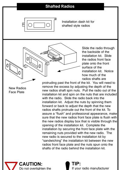
spin nuts securing the front face plate. Tighten to
