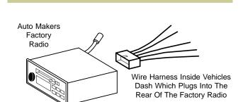
(Note: the radio shown is for display purposes and may not be similar in size or dimensions than the auto makers factory radio in your vehicle)
