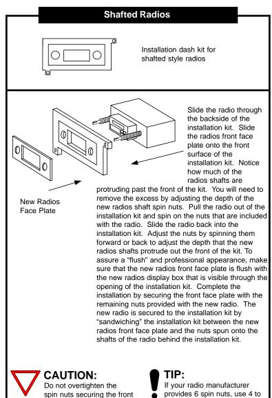
secure the radio to the installation kit and 2 to secure
