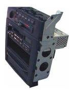
Nissan radio attached to the metal brackets and pocket below the radio
