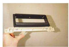
Picture shows the lower bracket originally attached to the GM radio mounted to the bottom of the radio installation kit.
