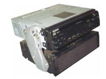
Insert the new radio into the metal brackets and secure the new radio with either the same screws that had secured the Nissan radio or the new radio should be packaged with 4 screws.
