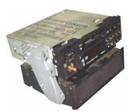
Nissan radio attached to pocket/ speaker below the radio by metal brackets on each side of the radio assembly.
