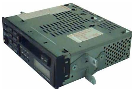
Nissan radio attached to the metal brackets and pocket below the radio
