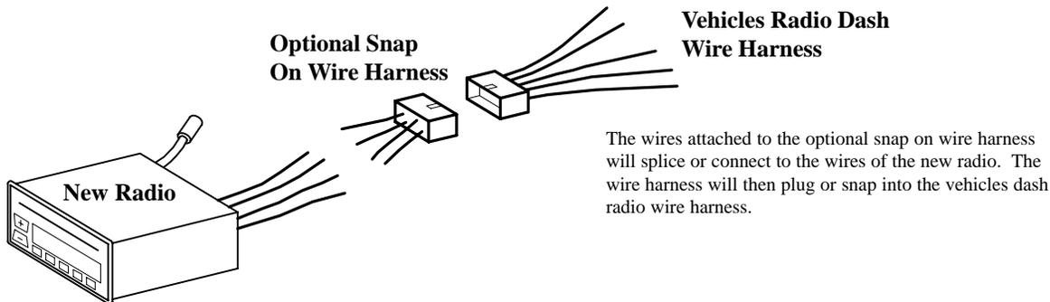
**DO NOT CUT OFF YOUR VEHICLES RADIO DASH WIRE HARNESS CONNECTOR** if possible. There are many advantages to leaving the vehicles radio in-dash wire harness connector attached to the wires. Here are some very important reasons:
