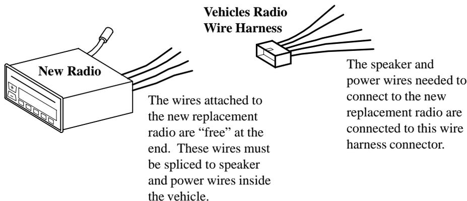
Until recently, in order for the “free” wire ends of the new radio to be spliced or connected to the wires attached to the vehicles indash radio wire harness, the vehicles wire harness connector had to be cut off, “freeing” the wires in the vehicles dash so that they could be spliced to the wires of the new radio.
