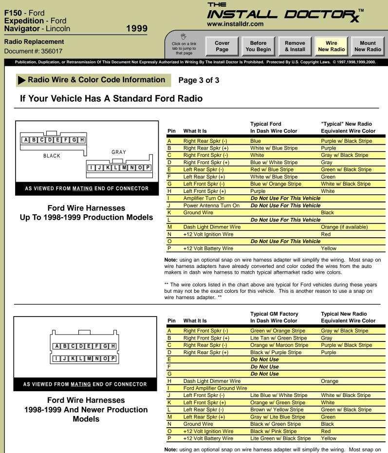
**Note:** using an optional snap on wire harness adapter will simplify the wiring. Most snap on wire harness adapters have already converted and color coded the wires from the auto makers in dash wire harness to match typical aftermarket radio wire colors.
