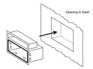
Push The Kit Into The Dash Opening Until It Snaps Into Place, Securing The Kit To The Dash.
