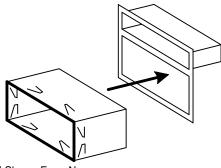
'DIN' Sleeve From New Replacement Radio
