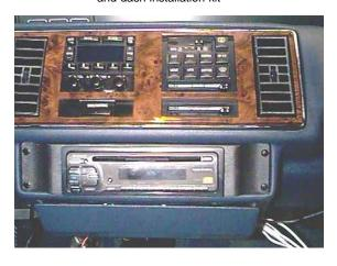
with dash installation kit and kit pocket in place of original radio display
