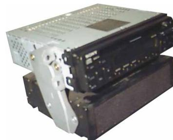
Insert the new radio into the metal brackets and secure the new radio with either the same screws that had secured the Nissan radio or the new radio should be packaged with 4 screws.
