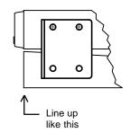
A common mistake when mounting your new radio to the auto makers radio bracket and pocket is selecting the wrong holes on the side of the new radio.
