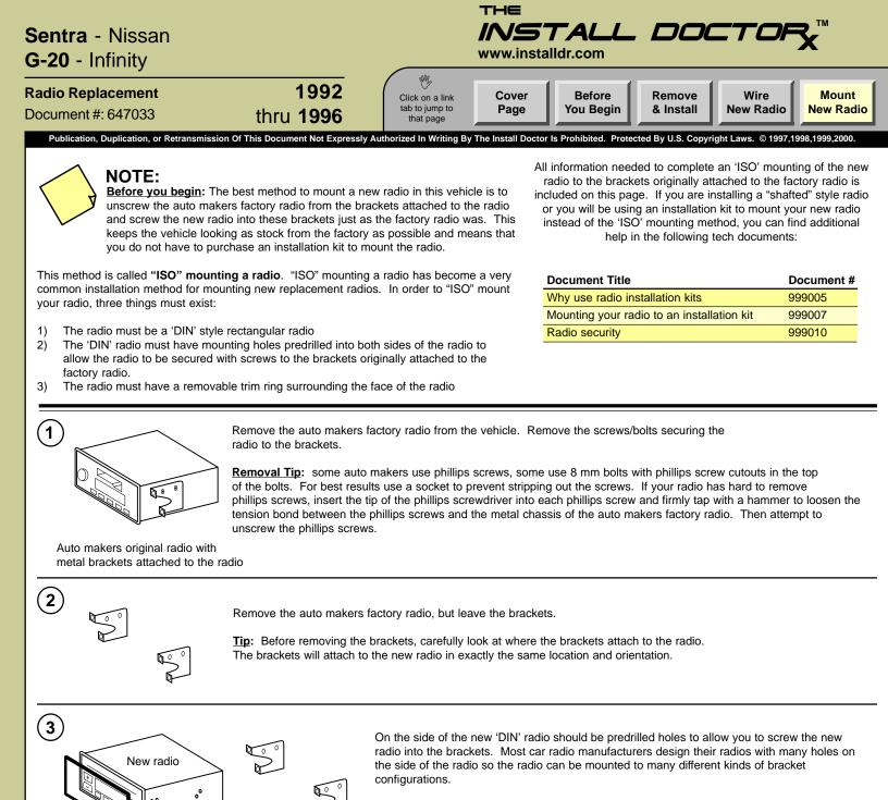
If you are going to mount your radio in this manner, you will probably have to remove the radios face trim ring around the face of the new radio. This trim ring will most likely prevent the vehicles dash panel from securing properly back onto the dash.
