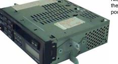
Nissan radio attached to the metal brackets and pocket below the radio
